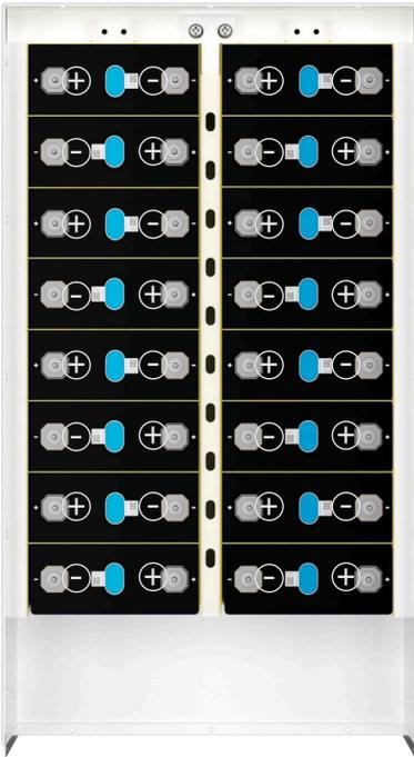
Place the battery cells in the chassis, separated by fiberglass insulation plate (K)
