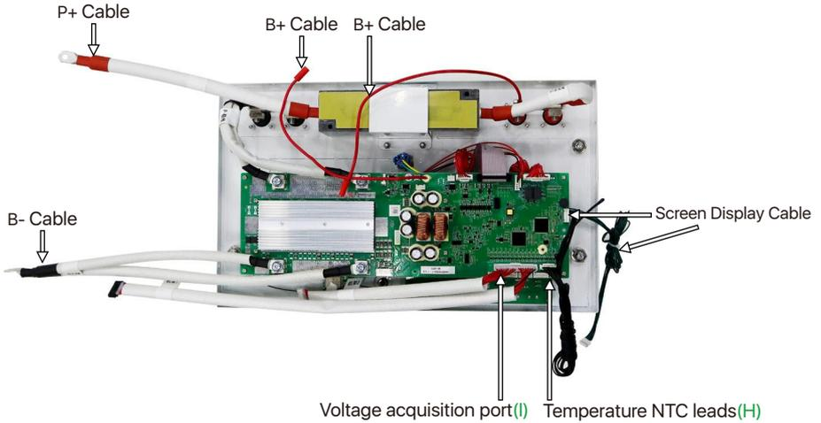
Check every connection, the voltage between the main positive and the negative is  $>52V$ , then turn the button on, the LCD and the indicator work out, then the assembly operation is completed.
