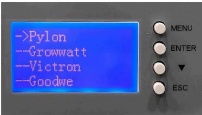
e. All of the indicators will light up after 3-5 seconds, and then it has a "bee" sound. The screen will show the latest communication protocol, which means the protocol has been updated successfully.
