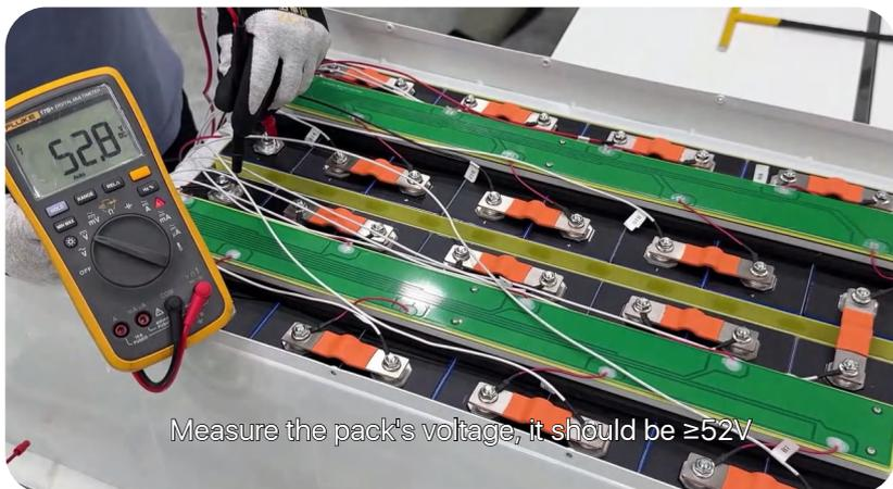
Measure the pack's voltage, it should be  $\geq 52V$
