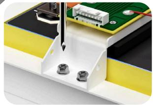
Link the PCB bars(C) and flexible busbar(M), then screw up(Torque: 5-6 Nm)
