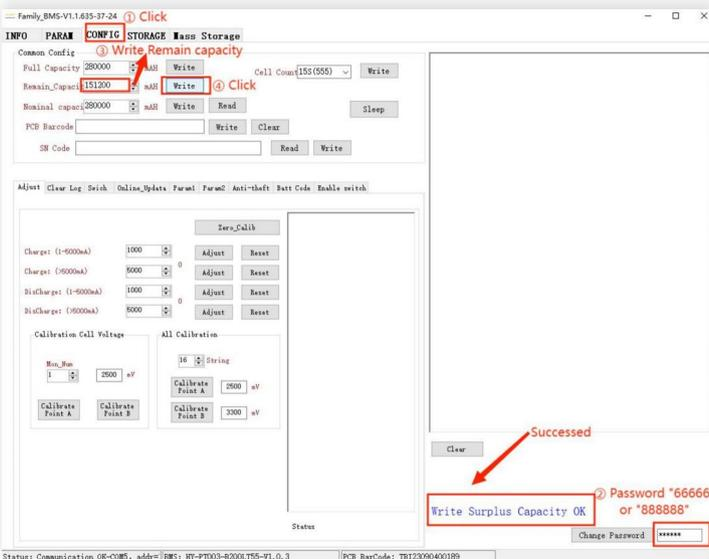
Important: After modifying the capacity, it is needed to perform a complete cycle(full charging and discharge) 1-2 times for the BMS to learn the latest status.
