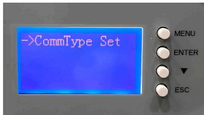
c. There are CAN/RS485 options, click the correct option based on the inverter model.
